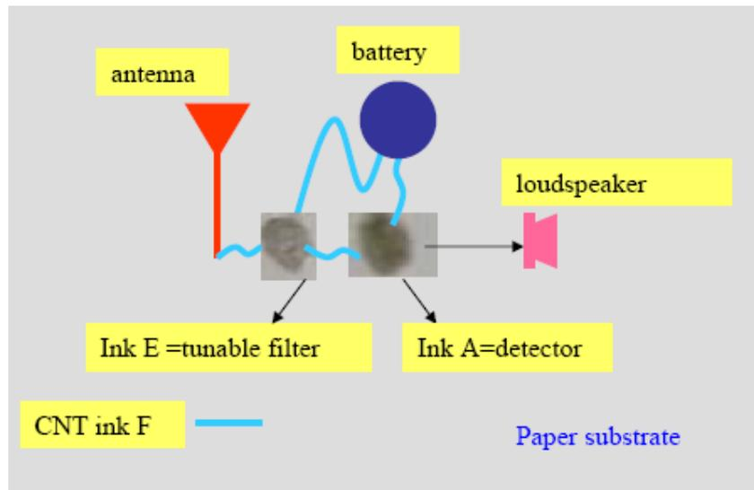
The radio on paper concept; CNT inks of various concentrations are used to implement various functions which are usually done by R, L, C components and copper.
