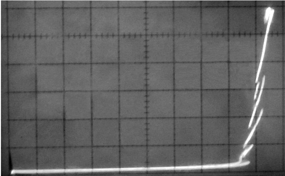
Multiple negative resistances at  $V_G = 14$  V, vertical :500  $\mu$ A/div, horizontal 2V/div
