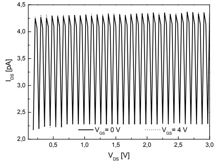
Drain current versus (a) negative and (b) positive drain voltage values, in the presence and absence of a gate voltage at room temperature.
