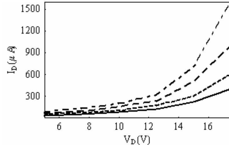
The  $I_D$ - $V_D$  dependence on the gate voltage for  $V_G = 0$  (solid line), 4 V (dotted line), 8 V (dashed line), and 12 V (dashed-dotted line).
